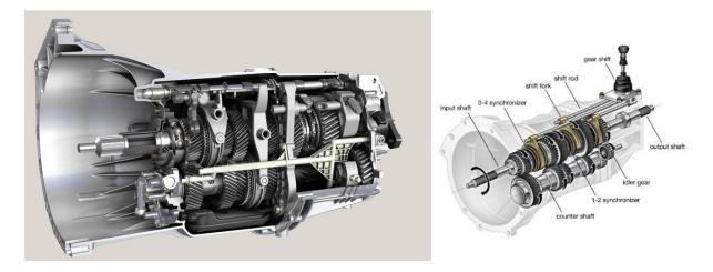
Figure 1 ZF 6 speed manual transmission together with a manual transmission schematic.
