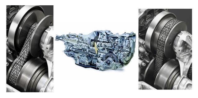
Figure 5 Subaru Linear Tronic CVT
