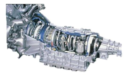
Figure 7 Nissan Extroid toroidal CVT
